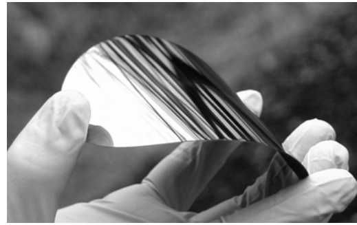
Fig. 5: 70 \mu\text{m} thin and flexible Ge wafer with solar cell structure.
