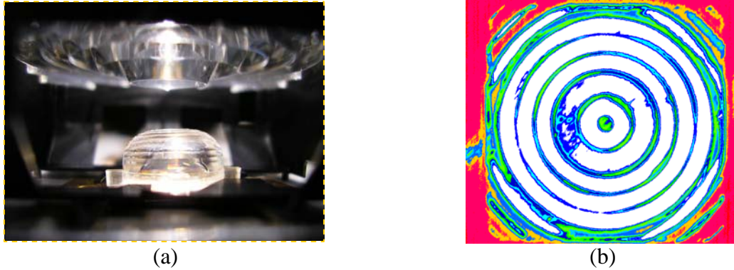
Fig. 5. (a) Compact concentrator being developed within the activity “manufacturing” (b) False colour picture of a test concentrator (front view). Blue regions indicate regions with poor transmission of light.
