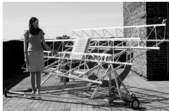
Figure 6: Photograph of the developed sun tracker for 1 kWp of installed capacity on the roof of the Ioffe Institute.
