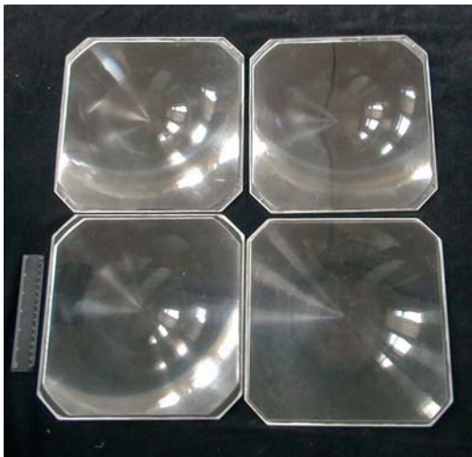
FIGURE 3. Fabricated Fresnel lenses with dimensions of 27cm x 27cm and focal distance of 30 cm designated for fabrication of 4 solar TPV modules.
