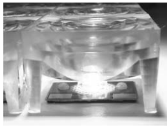
Figure 5. Photograph of a flat, non-imaging optics concentrating light energy onto a cell.
